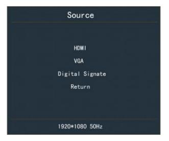
**HDMI**: Display the content from external HDMI signal port **VGA**: Display the content from external VGA signal port
